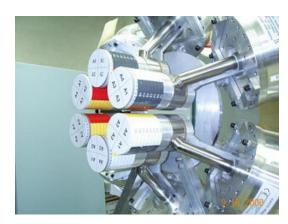
**miniSeGA**: A barrel of six close packed detectors (Inner diameter ~10.2 cm).
