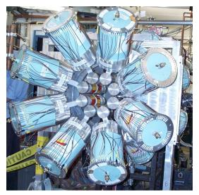
**betaSeGA**: 16 detectors in 2 rings surrounding beam line in a diameter of 17.3cm.
