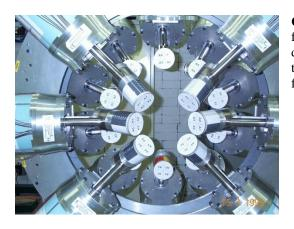
**ClassicSeGA**: Note that this photo only shows 6 detectors in the forward ring. The forward ring can accommodate up to 8 detectors (for 18 in the full array) except when run at the S800 target position where only 7 detectors can be placed in the forward ring.
