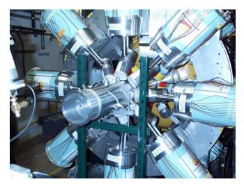
**plungerSeGA**: two rings of 8 detectors each at maximum forward (30°) and backward (140°) angle in order to obtain maximum Doppler shift of gamma lines for lifetime measurement in RDDS technique.
