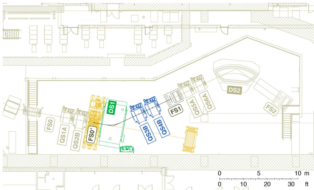
Figure 6-10 Layout of the neutron invariant-mass mode of the Spectrometer Section. The target station FS0' is located between QS2B and DS1.
